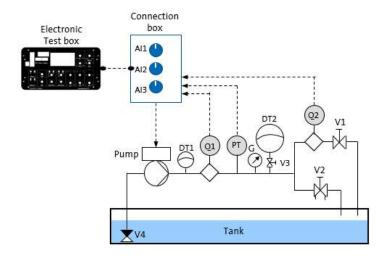
As seen from the drawings and the diagram, the standard CRNE demo consist of the following components:
