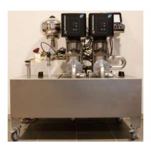
Pump 1 is connected to the Connection box having the possibility to use all three standard sensors. An extra pressure transmitter is mounted and connected directly to Pump 2.
